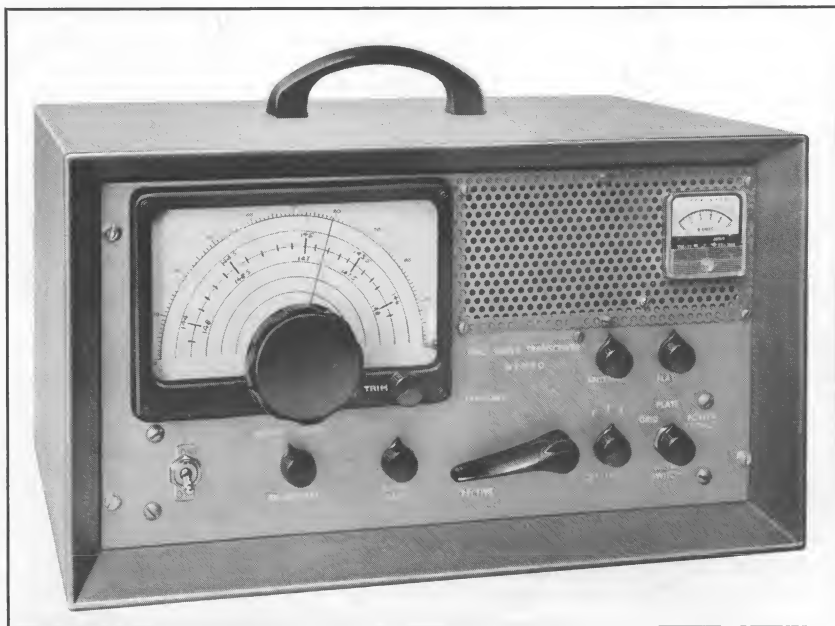
Figure 1: W2OKO's two-meter transceiver features large dial with vernier for easy tuning. All operating controls of the unit are located on the front panel.
